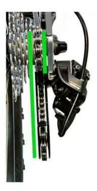
On each end, the high and low gear, there must be a way to limit how far the derailleur mechanism can travel. Otherwise, the derailleur can travel past the inner or outer chain ring and the chain will come off. This is done with limit screws. There will be small screws, generally marked H and L, on the derailleur. On both derailleurs, the L controls the low gears which are those closest to the bike. The H controls the high gears which are farthest from the bike.
